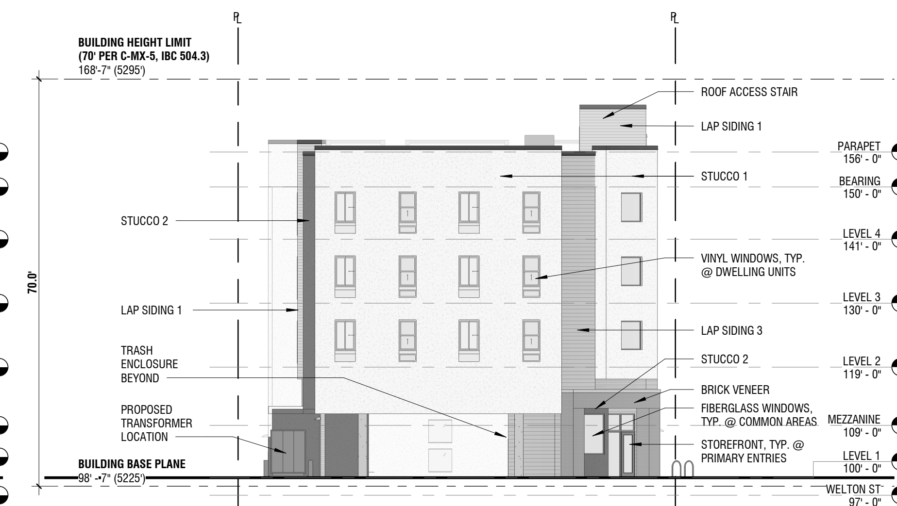
SOUTHEAST ELEVATION - PARKING ENTRANCE (ACCESS EASEMENT)
