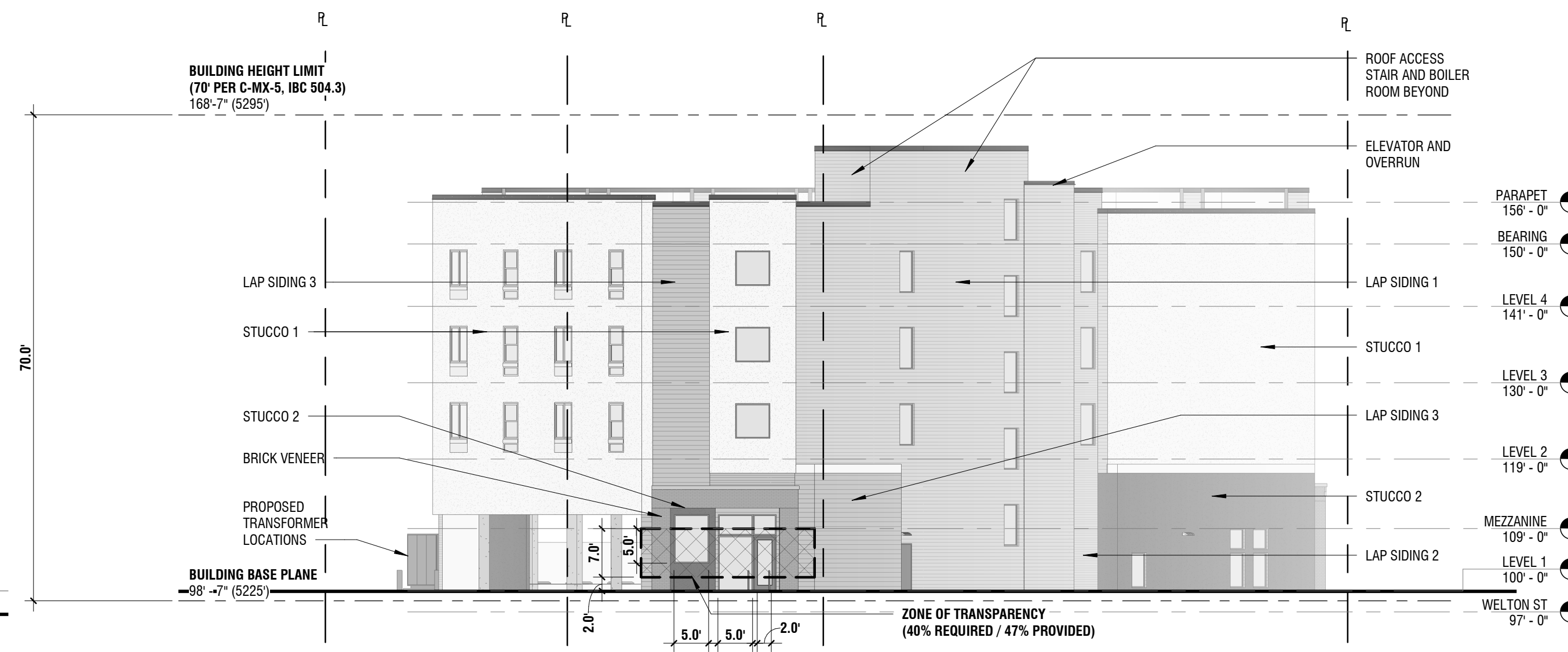
EAST ELEVATION - DOWNING ST. (PRIMARY STREET)
